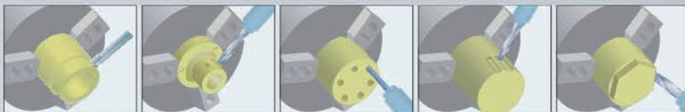
转弯 Turning 径向钻孔和攻丝 Radial Drilling and Tapping 端面钻孔和攻丝 End Face Drilling and Tapping 钻孔槽 Drilling Groove 轮廓加工 Contour Machining
