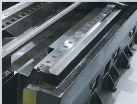
High rigidity roller type linear guides 高刚性滚柱式直线导轨
