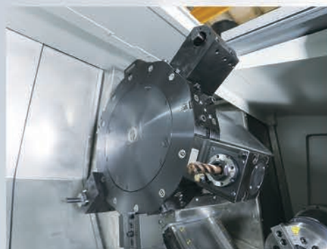
12/16 positions driven tools turret, all positions ready for driven tools
