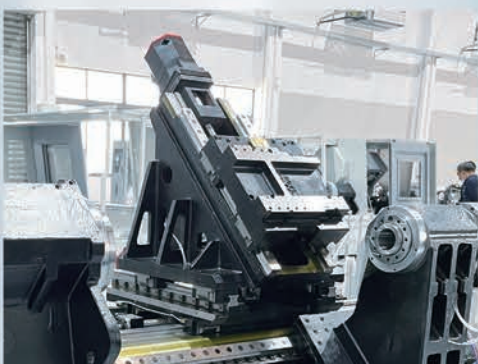
Super rigidity wedge structure Y axis 高刚性滚柱式直线导轨
